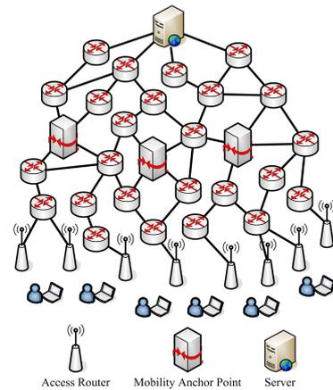
Fig. 1. A Typical Network Architecture of Hierarchical Mobile IPv6
