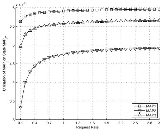
Fig. 6. Utilisation of  $MAP_j$  on State  $MAP_{j2}$  with Increasing Request Rate at All ARs in Scenario V
