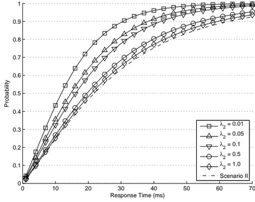
Fig. 5. CDF of the Response Time of AR1 in Scenario IV with Increasing Request Rate at AR2
