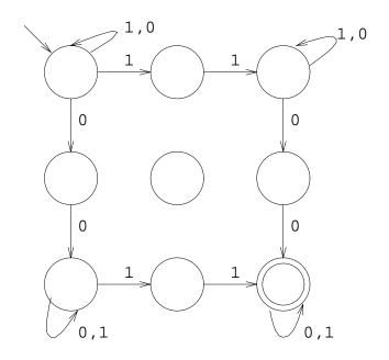
An acceptor FSM with  $\Sigma = \{0,1\}$  which accepts sequences containing two successive 0s and two successive 1s.
